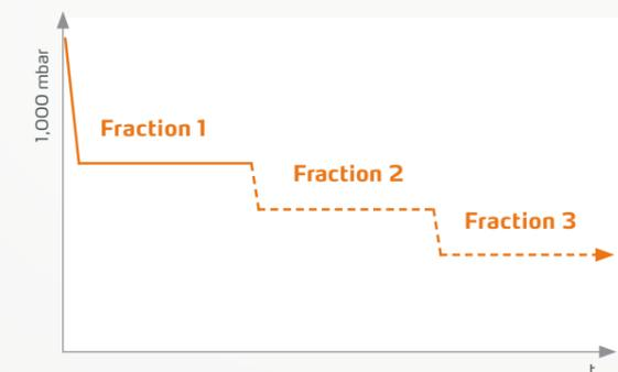
With DAA a completely automated distillation process can be started during the heating up phase of the heating bath. The system pressure is adjusted dynamically to the changing heating bath temperature, until the heating bath has reached the set temperature.
