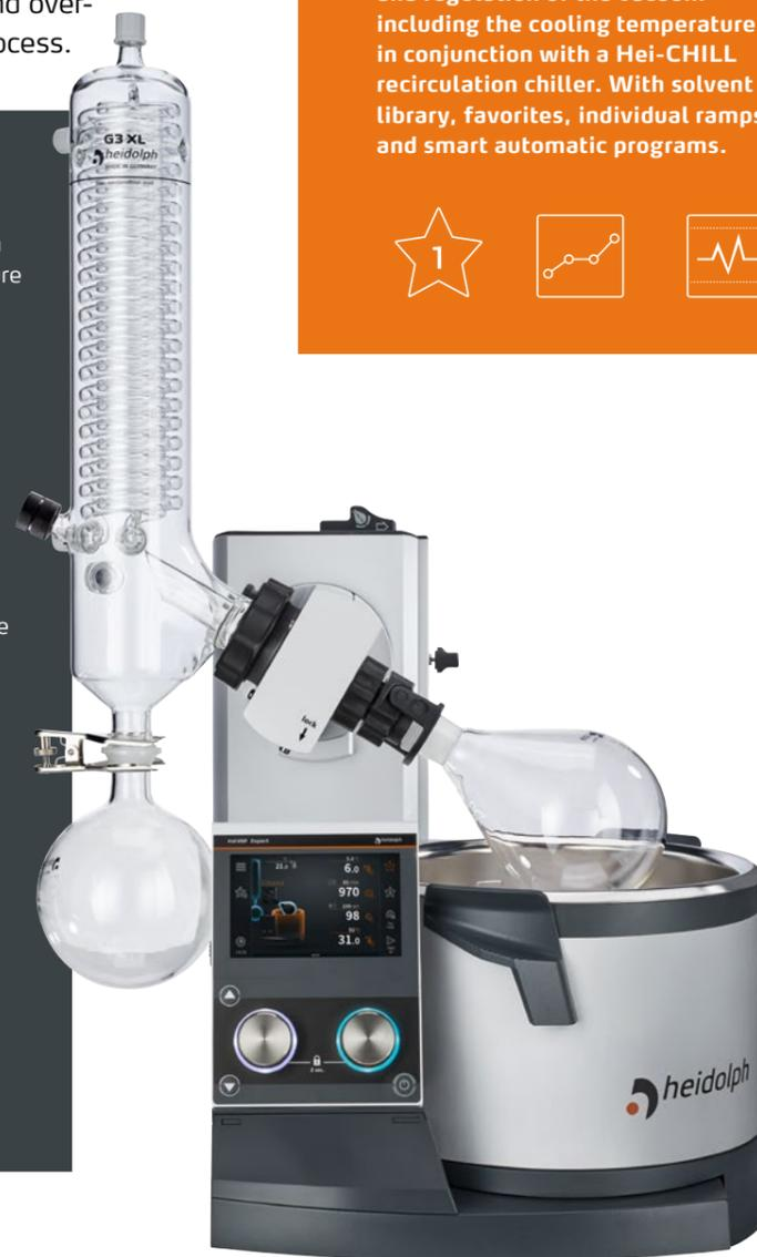
Control panel for central control and regulation of the vacuum – including the cooling temperature in conjunction with a Hei-CHILL recirculation chiller. With solvent library, favorites, individual ramps and smart automatic programs.
