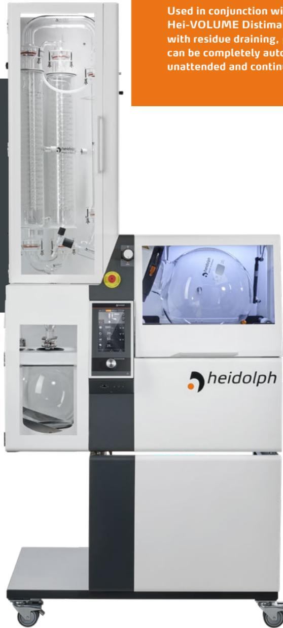
Used in conjunction with the automatic Hei-VOLUME Distimatic Pro module with residue draining, processes can be completely automated for unattended and continuous use, 24 / 7.
