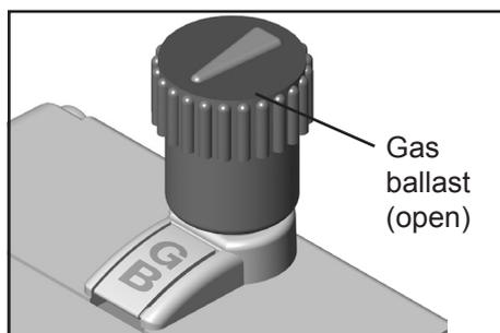
To reduce condensation in the pump, do not pump vapor before the pump has reached its operating temperature. Open the gas ballast valve when pumping condensable vapors.
