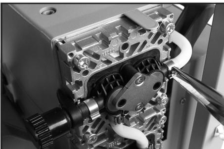
Affix the connection tube to the other side of the pump, as well as the hose connection to the inlet or outlet of the vacuum system at the valve head.
