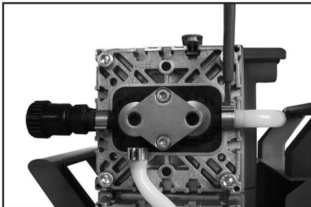
Detach the coupling of the connection tube to the other side of the pump as well as the hose connection to the inlet/outlet of the vacuum system at the valve head.
