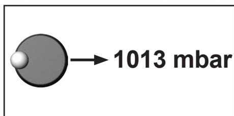
An adjustment at atmospheric pressure is only possible if the pressure is higher than 700 mbar.
