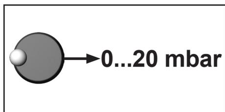
Instead of adjustment under vacuum to a pressure < 0.1 mbar, adjustment to a precisely known reference pressure within the range of 0 ..... 20 mbar is possible. Evacuate the measurement connection of the controller to a pressure within 0 ..... 20 mbar
