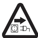
Isolate equipment from mains before removing the cover.
