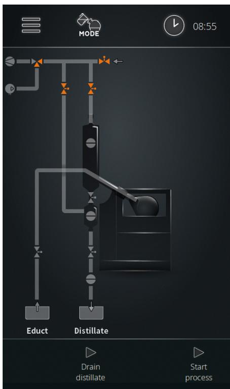
In manual mode, single batches can be processed. For automatic filling of the evaporation flask and draining of the distillate, the **Drain distillate** and **Start process** buttons are available on the operating panel.
