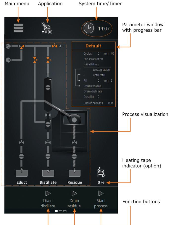
From the start window, you can access the main menu, select an operating mode directly, and select the time display.
