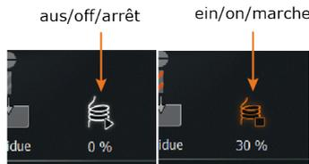
The operating behavior is defined by the process parameters of the selected mode (automatic switching on, on-period/pause time in percent).
