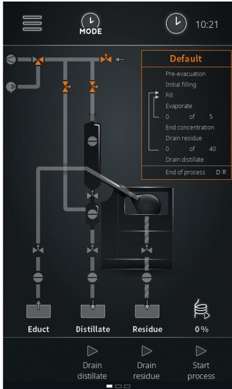
In the time mode, the filling of the evaporation flask, the distillation and the draining of the distillate and residue are carried out in a purely time-controlled manner:
