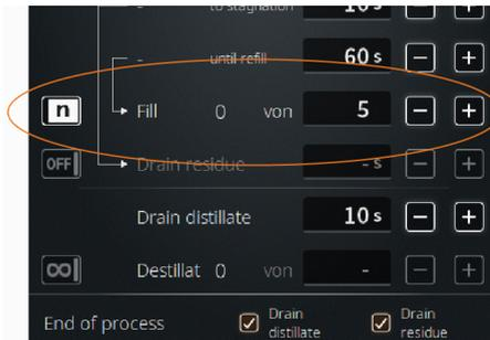
In the example: five fillings, then optionally an additional evaporation time runs. This allows a desired concentration to be achieved!
