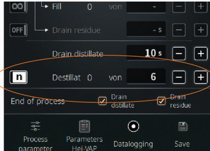
In the example: drain distillate six times, then the optional additional evaporation time runs. This allows a desired concentration to be achieved!
