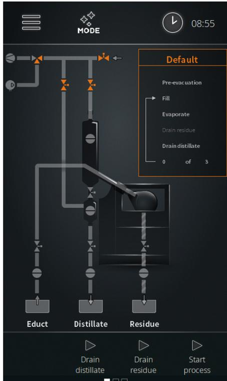
The rinse mode allows the fill and concentrate line to be flushed with a suitable solvent. The flushing process removes residues from previous processes and impurities. When rotation is activated, the evaporation flask is also cleaned.
