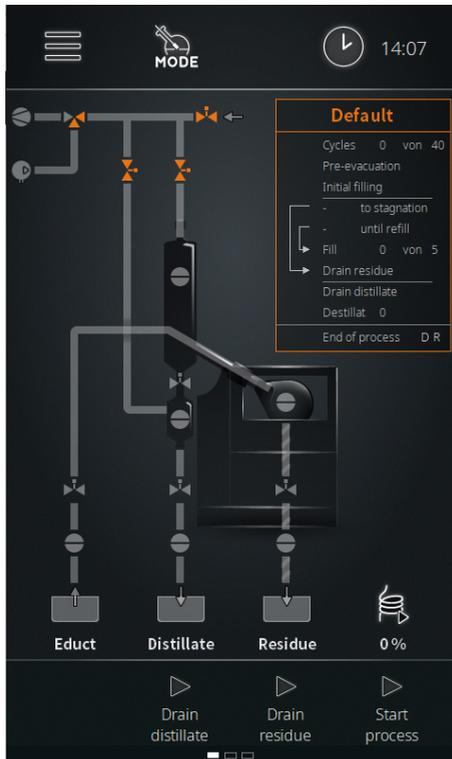
In sensor mode, the filling quantity in the evaporation flask is regulated by the flask level sensor S4. The following sensor statuses are possible:
