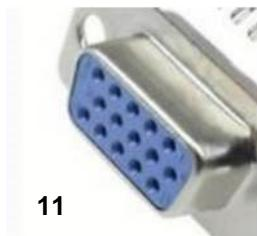
To connect your interface, you will need an interface cable with SUB-HDD 15 connector which fits the socket (11) located in the item's rear panel.
